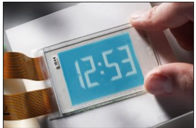
Fig 3 – Cyan clock with a 2.5" diagonal. The pixel resolution of the display is 160 ppi.
