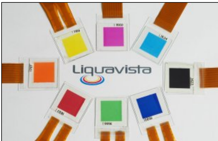
Fig 1 – A sample of the brilliant colors that can be made with the electrowetting display technology. By varying the dye dissolved in the oil, an unlimited range of colors can be provided.
