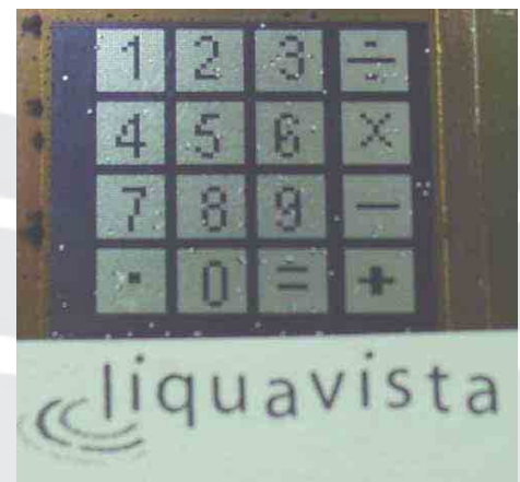
Figure 12 – Active matrix addressed electrowetting display. The logo at the bottom off the figure is printed on paper to illustrate the reflective performance of the electrowetting display
